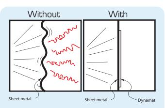
Sheet metal subjected to impact creates noise. With Dynamat installed, the noise is transformed into silent energy through a process called "Vibro-Acoustic Energy Conversion". Dynamat converts the vibrational energy into low-grade thermal energy. The result is a more quiet and comfortable living environment.
